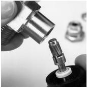
**Note:** If the insert shows signs of wear or damage it must be replaced.
