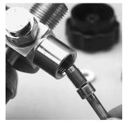
**Note:** If the insert being installed is new then apply a thin film of christo-lube lubricant to the threads of the insert before assembling.
